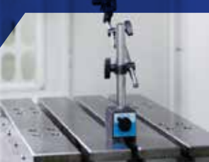
4. Spindle deflection test
