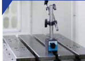
4. Spindle deflection test
